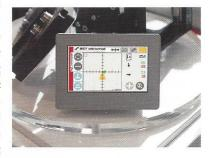
tors, speed up the setup process and reduce waste. With RegiTouch, machine operators can quickly and easily move the register marks for the printing units, which need to be guided to the required positions either during make-ready or after non-format-related roll changes. All operators need to do is select the register marks for the individual colors on the regi\_star 20 touchscreen and move them into a defined area.
